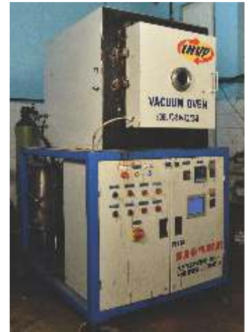
Fig. 1 Microprocessor controlled heating chamber used for producing thermally modified wood in the laboratory
