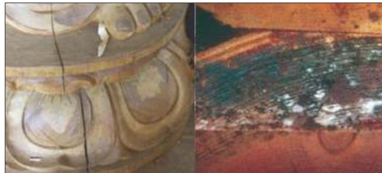
Fig. 2. Cracks and fungal growth in poorly seasoned wooden products
