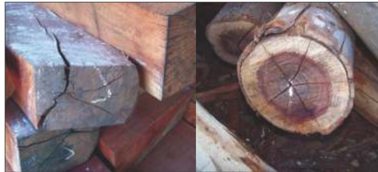
Fig. 1. End cracks in sawn slabs and logs of wood
