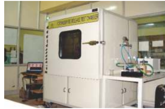
Fig. 4. Small chamber of 1 M3 established at IPIRTI for steady state formaldehyde emission aggressively regulated. The California Air Resources Board (CARB) recently established a new set of product emission control measures. CARB's two-step process tightens allowable formaldehyde emissions from raw composite wood panels (particleboard, medium density fiberboard and hardwood plywood) and all products constructed out of them (such as flush doors).
