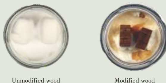
Fig. 3 Rubberwood specimens exposed to white-rot ( Tremetes hirsuta ) after 16 weeks of exposure.
