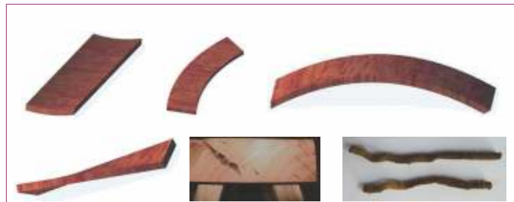
Fig. 6. Defects in timber due to improper seasoning
